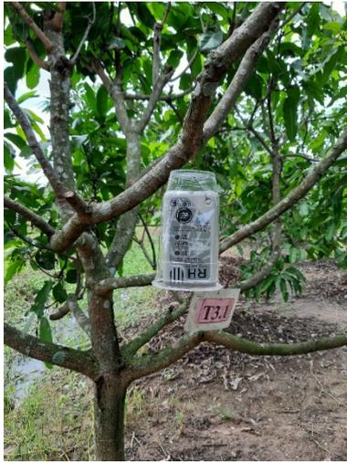
**Figure 4. Temprecord RH humidity and temperature logger**
