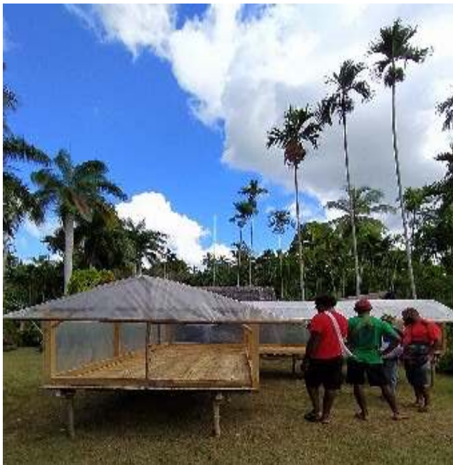
Figure 5: Simple design solar drier in Hobe Village, Madang District, modified from an Outspan model with clear plastic covering; farmers are using their own initiative to modify the basic design.
