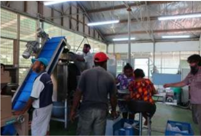
Figure 1: The new crew working with Equanut, the private sector partner using mechanical cracker to crack nut in shells.
