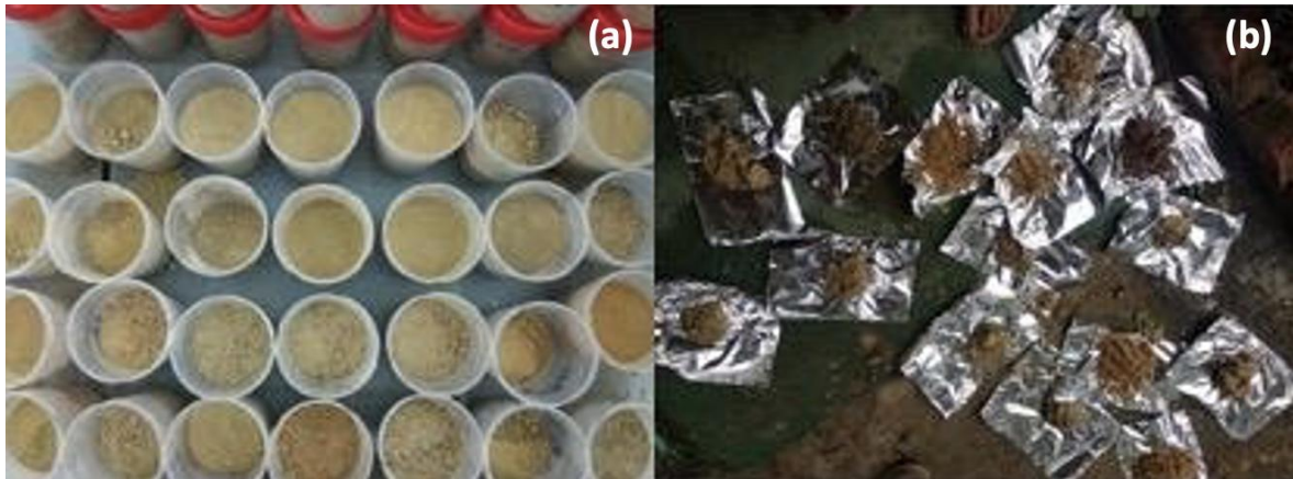
Figure 3: Soil samples collected during the borewell construction: (a) sieved sample (b) original sample
