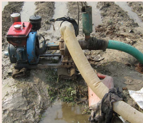
Small diesel-powered pump used to irrigate fields before planting crops, Bhagalpur, Bihar, India, 2012. Photo: Peter Brown, CSIRO
