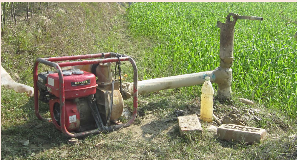
Small diesel-powered pump used to irrigate wheat fields, Dhanusha, Nepal Terai, 2015. Photo: Peter Brown, CSIRO
