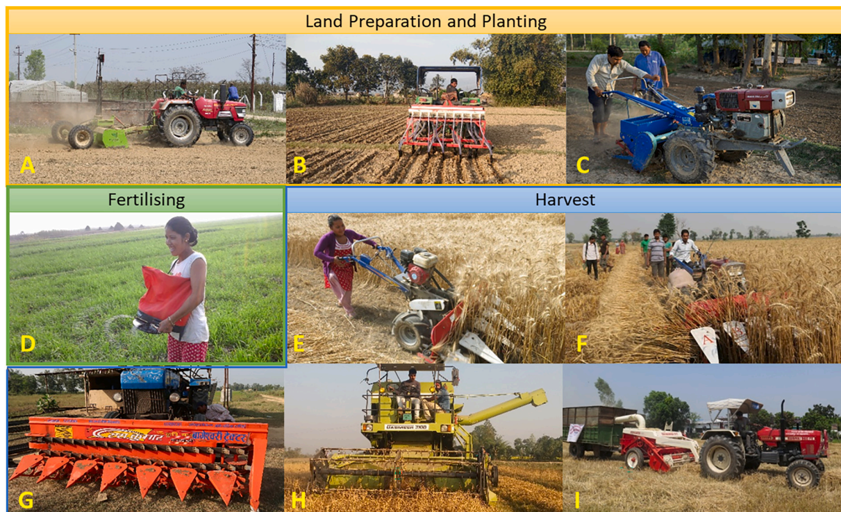
Fig. 1. Nine 'sustainable intensification' agricultural mechanisation technologies investigated in this study: [A] Laser Land Leveller; [B] four-wheel tractor (4WT) seed drill; [C] a two-wheeled (2WT) seed drill; [D] Fertilizer Spreader; [E] Self Propelled Reaper; [F] 2WT attachable reaper; [G] 4WT attachable reaper; [H] Combine Harvester; and [I] Bhusa Straw Reaper. Photo Credit: CSISA Project team/CIMMYT.
