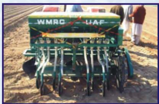
Bed planter that plants the seed and at the same time apply fertilizer
