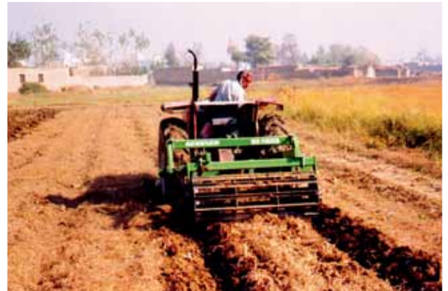
An Australian machine in Mardan, Pakistan, renovates beds on which maize was grown. The undisturbed stalks of the previous crop and seeds on the bed surface illustrate the retention of root systems and lack of soil inversion.
