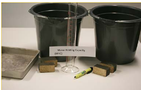
Figure 3.5 Equipment for the WHC and AFP tests.
