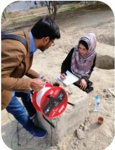
New piezometers (observation wells) with continuous logging are installed in community spaces in all case study areas. They are generating quality data for modelling, and provide a focal point for local capacity building re groundwater.
